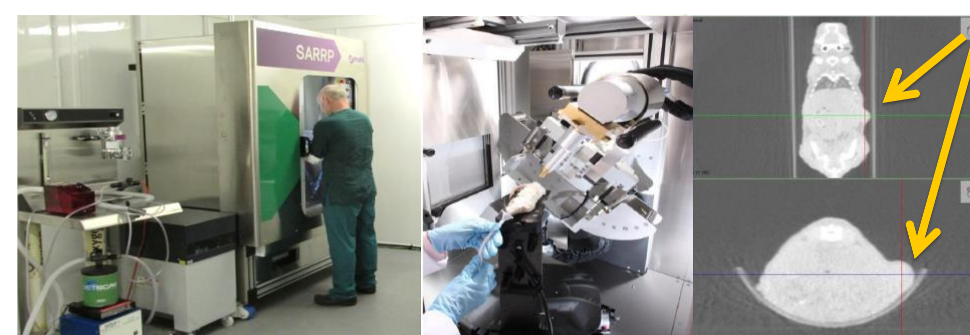
Figure 1: External view of SARRP (left), internal view showing robotic stage, rotating gantry and X-ray tube (middle), isocentre identification using MuriSlice software with CT imaging (right)
